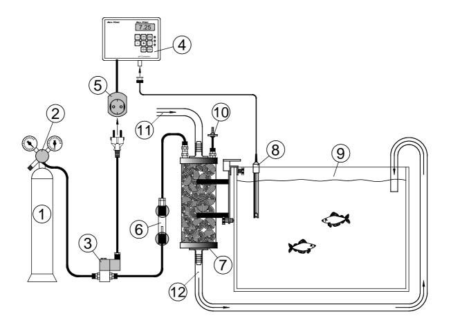
figu. 2: reactor 1000 on aquarium with automatic CO2 control
